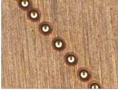
Fine spot welding of copper material (200 \mu m)
