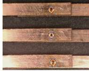
Welding of bus bars made of 0.2mm thick copper plates
