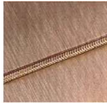
Butt welding of copper materials
